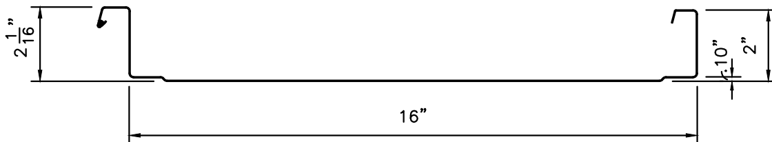
216 Roof Panel With Flat Pan
